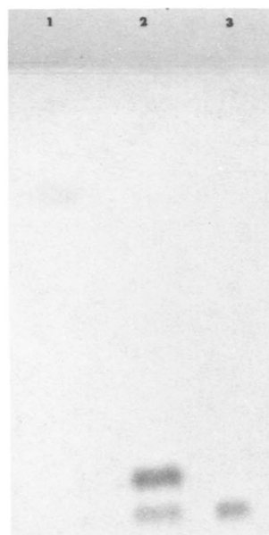
Fig. 3. Thin-layer chromatogram of native fraction 1 (lane 1) and fraction 1 after alkaline hydrolysis (lane 3). Lane 2, mixture of 7\alpha -hydroxycholesterol (lower spot) and 7\beta -hydroxycholesterol (upper spot). Solvent system, ethyl ether–water 100:0.5.
